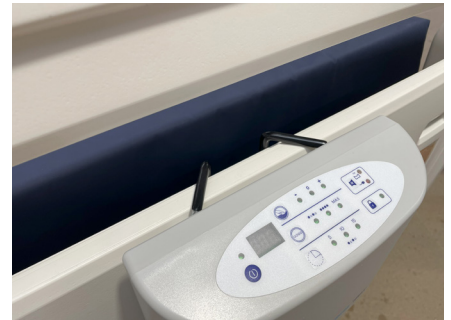
Hanging of control unit brackets
