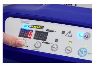
The immersion scale and pressure monitor shows live feedback to the caregiver on pressures inside the mattress. This may change as the patient moves position and can help detect when optimum immersion is achieved.
