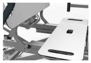
The backrest regresses as it lifts to 70°, lengthening the platform by 12cm, which reduces slipping thus reducing shear and friction and maximising comfort.
