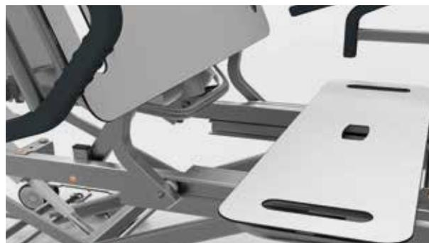
The backrest regresses as it lifts to 70°, lengthening the platform by 12cm, which reduces slipping thus reducing shear and friction and maximising comfort.
