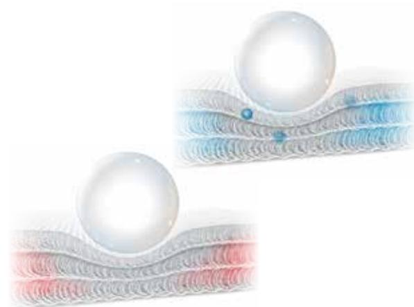
In contrast to foam, gel and air cells, the textiles inside AeroSpacer comprise an open, breathable structure, removing heat and humidity at the skin/
